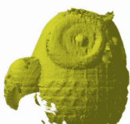
Scanning result of a translucent object
